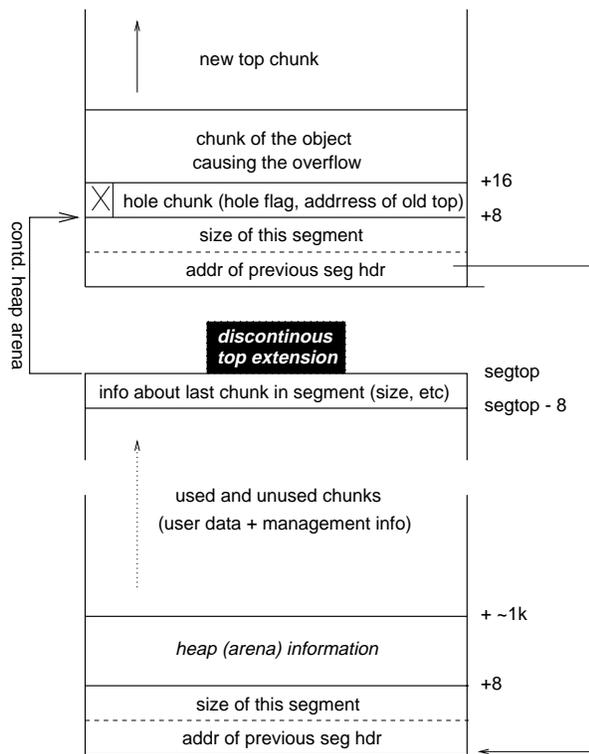
Figure 5: Heap extension
