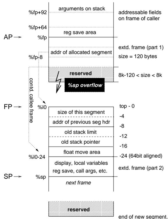
Figure 4: Non-linear stack extension
