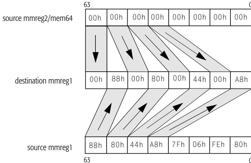
In the functional illustration of the PUNPCKHBW instruction, the 8-bit values from mmreg1 are stored in the low-order 8 bits of the 16-bit result. The mmreg2/mem64 source operand is set to all zero bits so it can provide zero fill in the high-order 8 bits of the 16-bit result. This is a method that can be used to expand unsigned 8-bit values into unsigned 16-bit operands for subsequent processing that requires higher precision.
