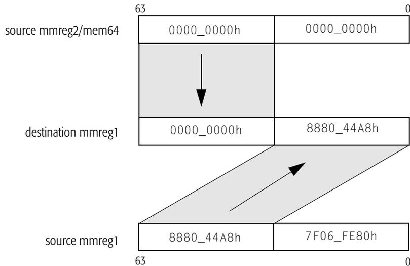
In the functional illustration of the PUNPCKHDQ instruction, the 32-bit value from mmreg1 is stored in the low-order 32 bits of the 64-bit result. The mmreg2/mem64 source operand is set to all zero bits so it can provide zero fill in the high-order 32 bits of the 64-bit result. This is a method that can be used to expand unsigned 32-bit values into unsigned 64-bit operands for subsequent processing that requires higher precision.
