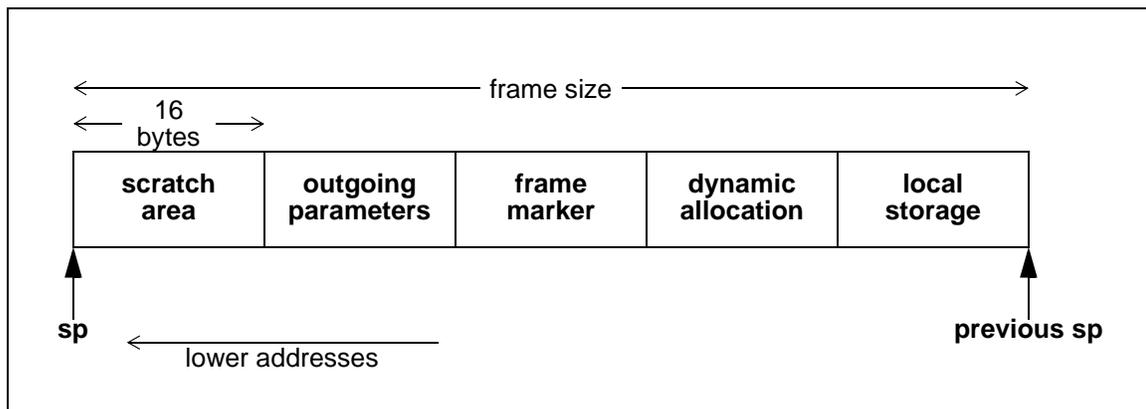
**Figure 7-1. Procedure frame**
