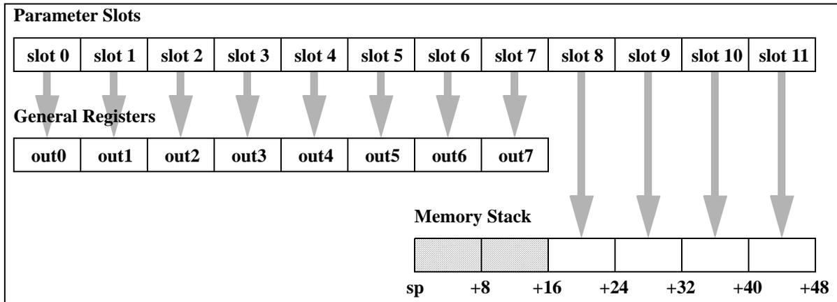
Figure 8-3. Parameter Passing in General Registers and Memory
