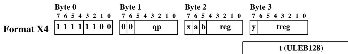
This format is used only by the *spill\_reg\_p* descriptor record, which identifies when a register is saved to another register under control of a predicate, or when a register is restored under control of a predicate.
