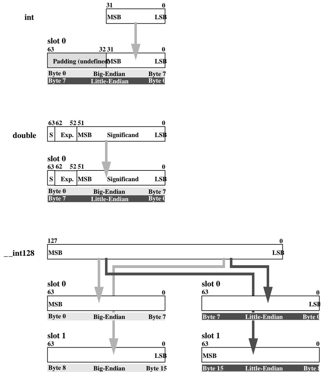
Figure 8-4. Examples of “LSB” Alignment
