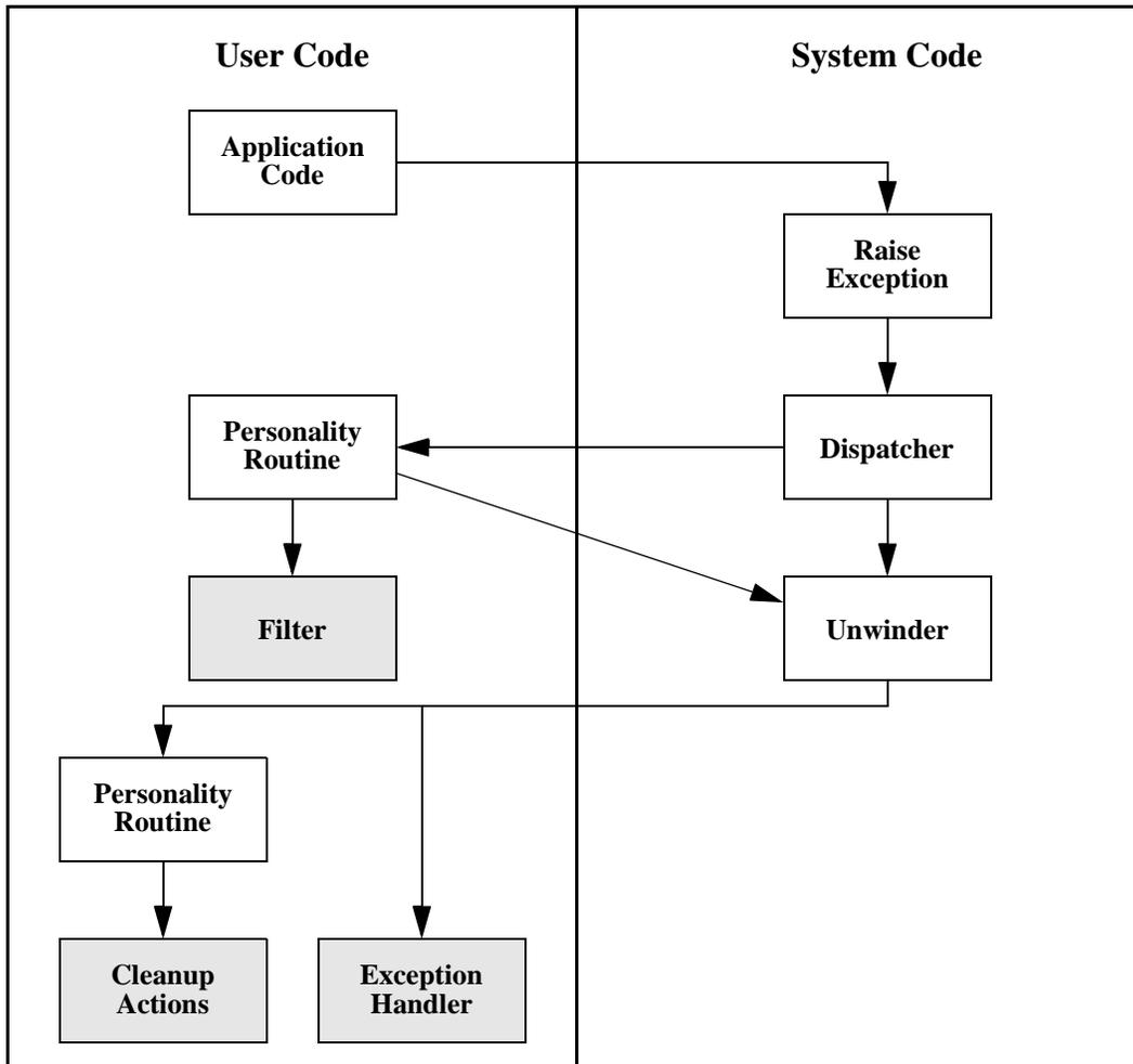
Figure 11-1. Components of the exception handling mechanism
