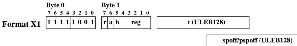
This format is used by the `spill_psprel` and `spill_sprel` descriptor records, which identify when a register is saved by spilling to the memory stack. The `r` bit identifies the record type, as shown in the following table:
