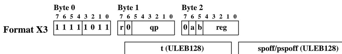
This format is used by the *spill\_psprel\_p* and *spill\_sprel\_p* descriptor records, which identify when a register is saved under control of a predicate. The *r* bit identifies the record type, as shown in the following table:
