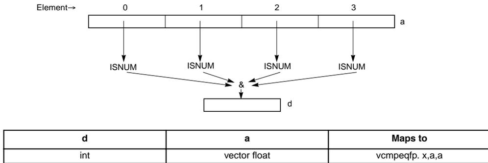
**Figure 4-179. All Numeric of Four Floating-Point Elements (32-Bit)**
