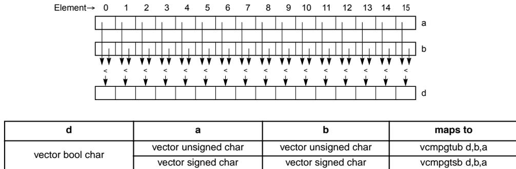
**Figure 4-37. Compare Less-Than of Sixteen Integer Elements (8-bits)**
