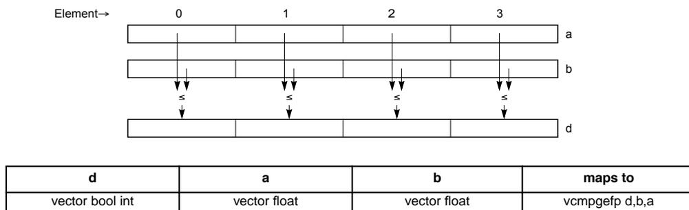
**Figure 4-36. Compare Less-Than-or-Equal of Four Floating-Point Elements (32-Bit)**
