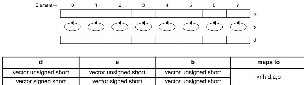
**Figure 4-98. Left Rotate of Eight Integer Elements (16-bit)**
