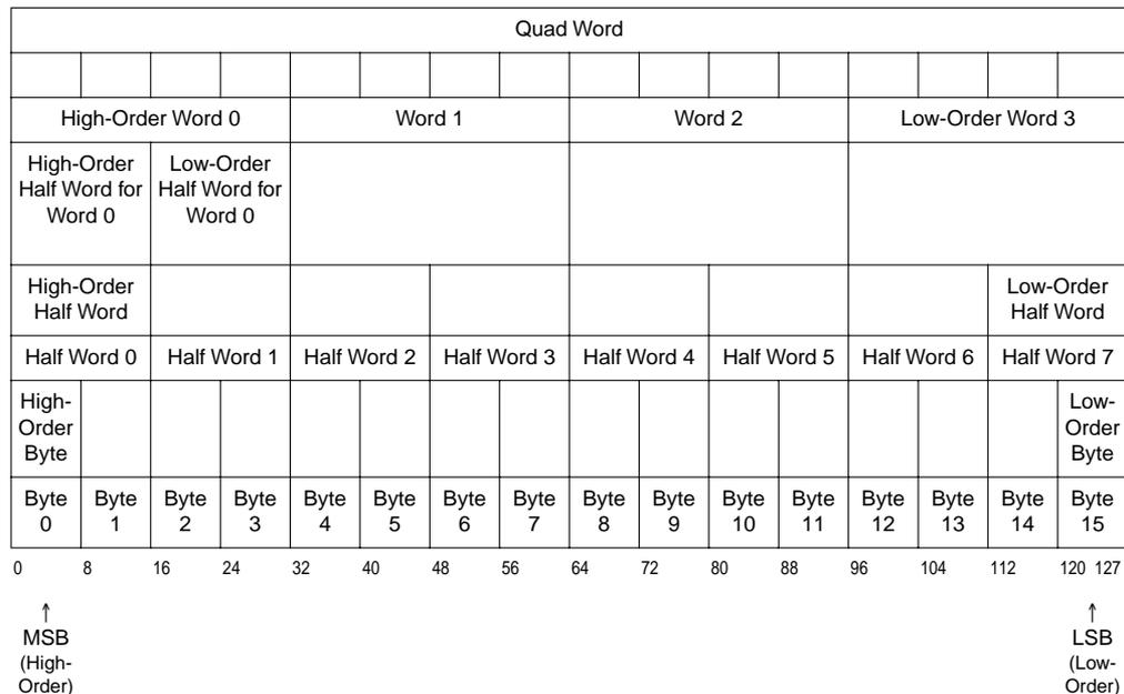
**Figure 4-3. Big-Endian Byte Ordering for a Vector Register**
