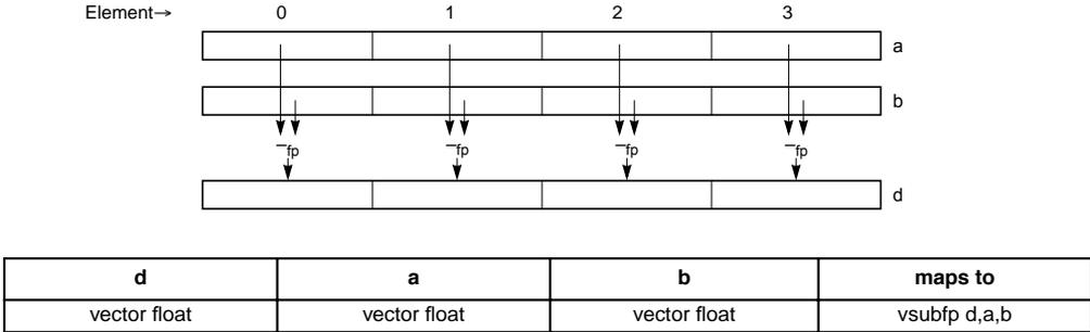
Figure 4-132. Subtract Four Floating-Point Elements (32-bit)
