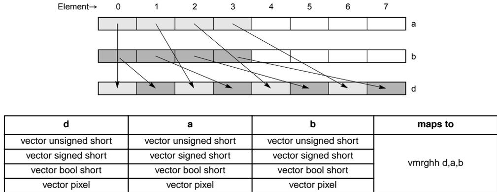
**Figure 4-65. Merge Four High-Order Elements (16-bit)**
