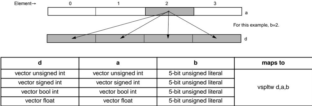
**Figure 4-111. Copy Contents to Four Integer Elements (32-Bit)**
