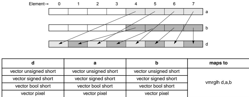
**Figure 4-68. Merge Four Low-Order Elements (16-bit)**
