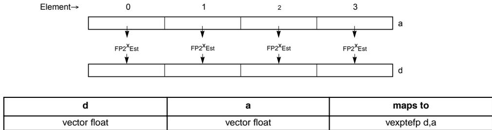
**Figure 4-52. 2 Raised to the Exponent Estimate Floating-Point for Four Floating-Point Elements (32-Bit)**
