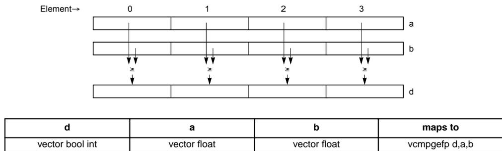
**Figure 4-31. Compare Greater-Than-or-Equal of Four Floating-Point Elements (32-Bit)**
