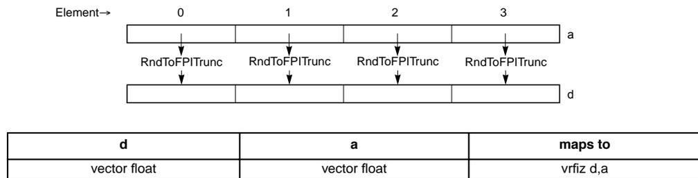
**Figure 4-141. Round-to-Zero of Four Floating-Point Integer Elements (32-Bit)**
