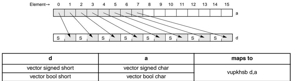
**Figure 4-142. Unpack High-Order Elements (8-Bit) to Elements (16-Bit)**
