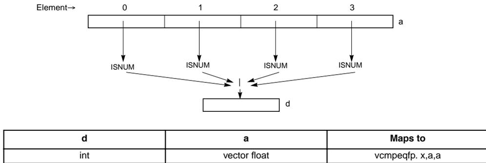
**Figure 4-209. Any Numeric of Four Floating-Point Elements (32-Bit)**
