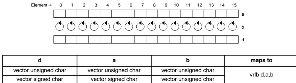
**Figure 4-97. Left Rotate of Sixteen Integer Elements (8-Bit)**
