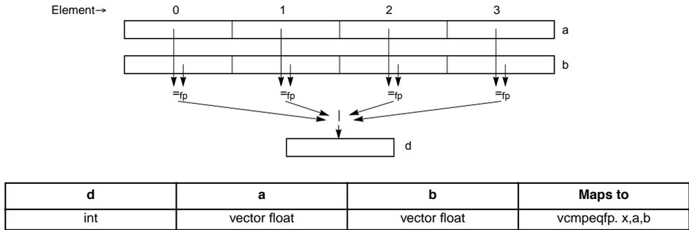
**Figure 4-183. Any Equal of Four Floating-Point Elements (32-Bit)**
