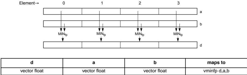
**Figure 4-74. Minimum of Four Floating-Point Elements (32-bit)**
