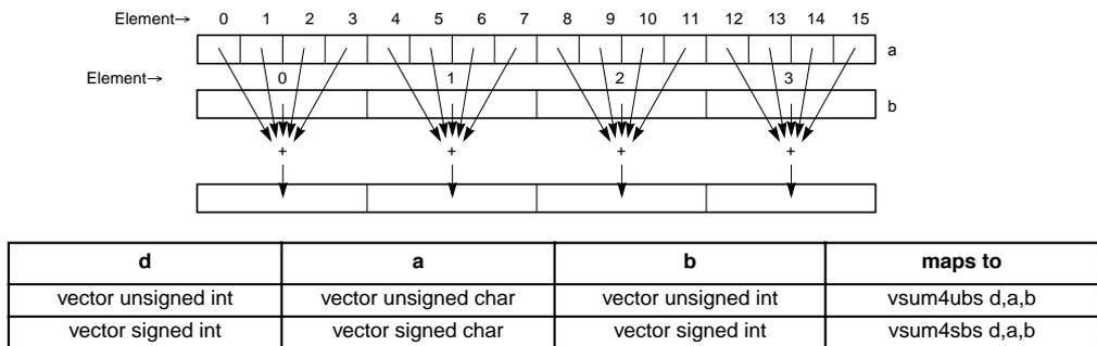
Figure 4-137. Four Sums in the Integer Elements (32-Bit)
