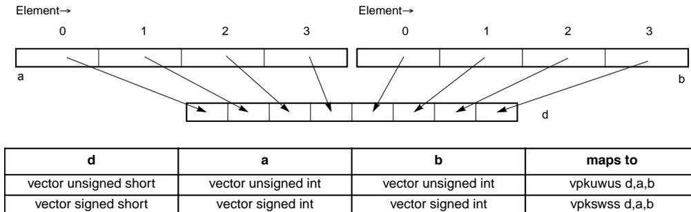
**Figure 4-92. Pack Eight Integer Elements (32-Bit) to Eight Integer Elements (16-Bit)**
