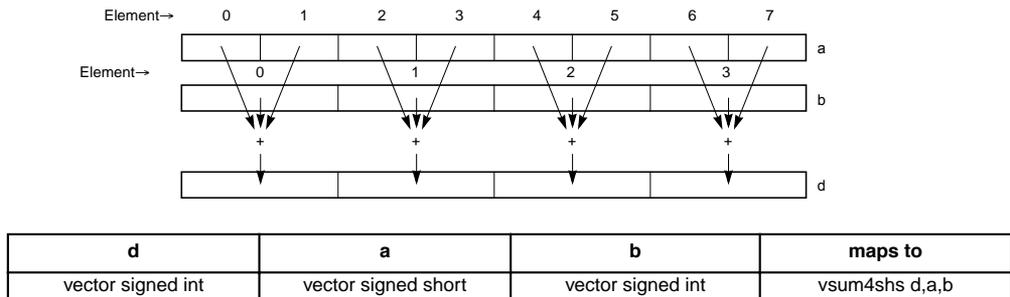
Figure 4-138. Four Sums in the Integer Elements (32-Bit)
