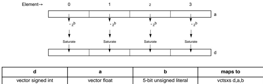
**Figure 4-42. Convert Four Floating-Point Elements to Four Saturated Signed Integer Elements (32-Bit)**
