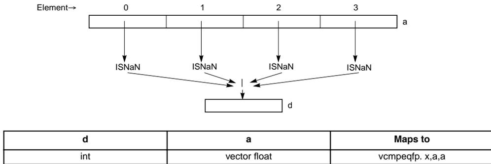
**Figure 4-200. Any NaN of Four Floating-Point Elements (32-Bit)**
