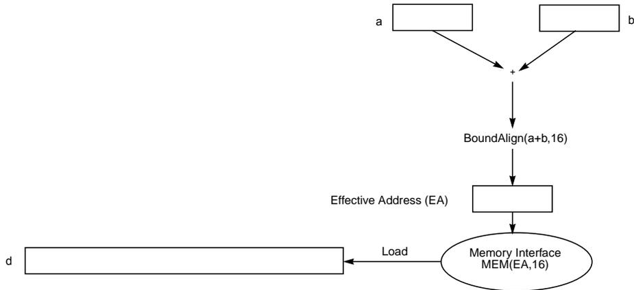
**Figure 4-54. Vector Load Indexed Operation**
