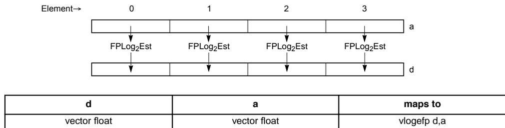
**Figure 4-57. Log<sub>2</sub> Estimate Floating-Point for Four Floating-Point Elements (32-Bit)**
