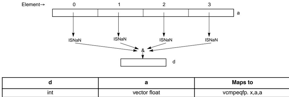
**Figure 4-170. All NaN of Four Floating-Point Elements (32-Bit)**
