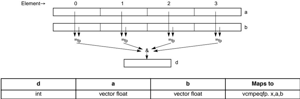
Figure 4-152. All Equal of Four Floating-Point Elements (32-Bit)
