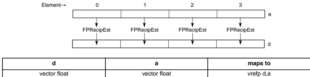
**Figure 4-96. Reciprocal Estimate of Four Floating-Point Elements (32-Bit)**
